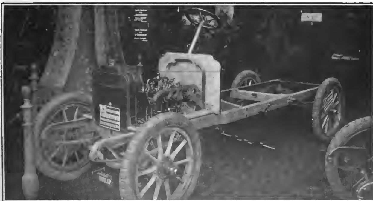
FIG. 5.—CHASSIS OF PRIMA FOUR-CYLINDER SMALL CAR AS EXHIBITED AT THE PARIS SALON.
